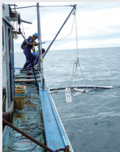
Left: Marine electromagnetic (EM) system in a shallow-water environment. Right: Deployment of the EM system from a boat.
