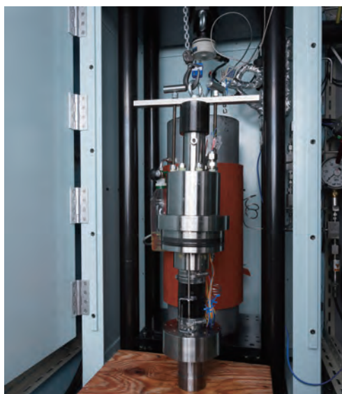
Left: Experimental setup for high-pressure fluid flow tests in a supercritical CO 2 -water system.
