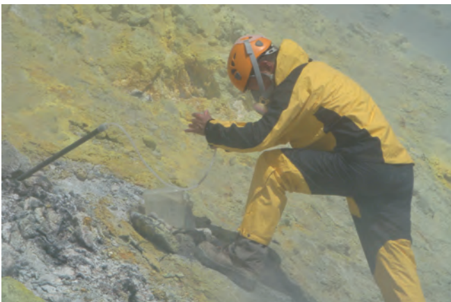
Left: Sampling of high-temperature (800 °C) volcanic gases into a vacuum glass bottle at Satsuma-Iwojima Volcano.
