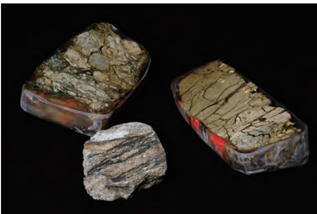
Left: Polished slabs of fault rocks used to develop new criteria for fault activity evaluation.
