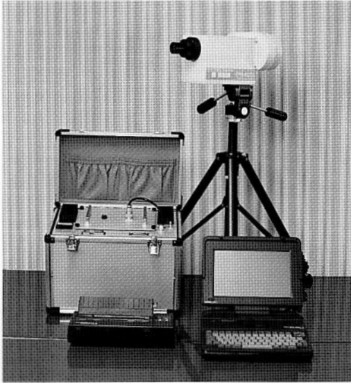
1 A field unit of the radiometer. An optical head on the tripod, a control unit (left), and a lap-top computer (bottom right) with a printer (bottom left).
