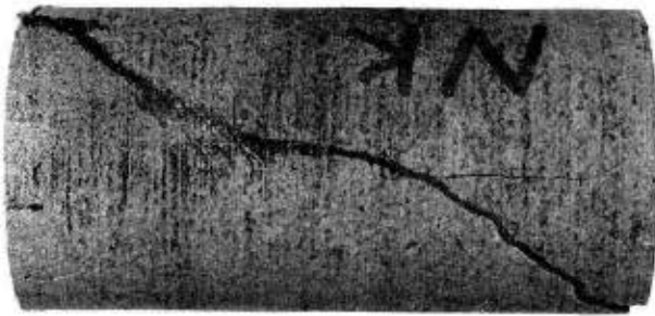
NK10, deformed at 1 kg/cm 2 . A strong fracture seems to be a kind of shear fracture. However, an extension-like fracture that extends from a curving point of the shear fracture might be very interesting for the understanding of fracturing mechanism of this specimen.
