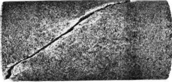
HSF 4, deformed at 1500 kg/cm 2 . Single shear fracture with network deformation bands inside the specimen.
