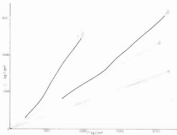
Fig. 236 Angle of fractures for pyroclastic rocks on \sigma - \tau co-ordinate.
