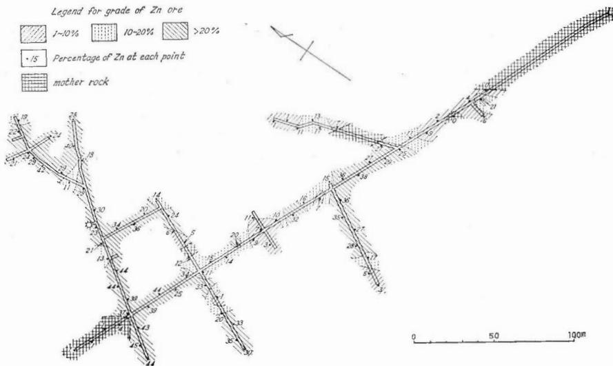
Fig. 12 Assay map for Zinc in Tunnel I.
