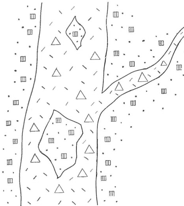
Fig. 14 Differences of crystal habits of pyrite between in vein and in mother rock (Udo mine)
