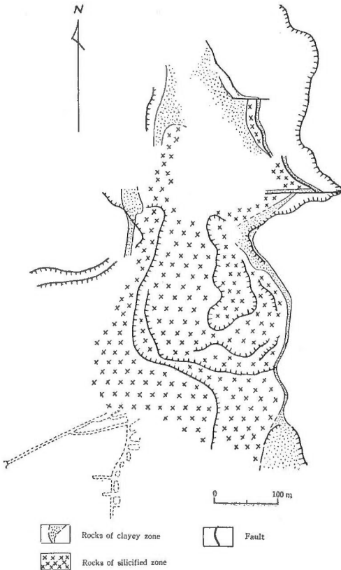
Fig. 4 Map showing the distribution of the altered rocks at the open pit of the Kosaka mine
