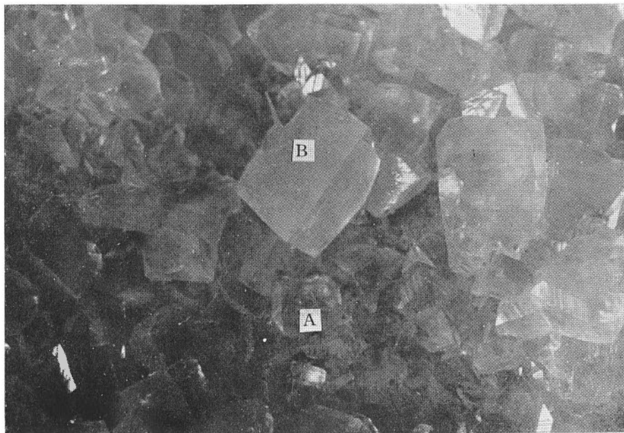
A photograph of specimen type 7 (Fukuhara). Showing the habit 6 crystals of the earlier crystallization (A) with small or middle developed +S face, and of the later crystallization (B) without +S face.
