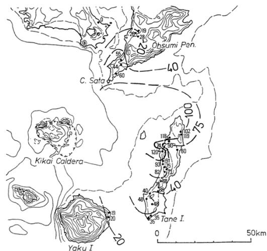
Fig. 4 Isopach map for the Ns-1 pyroclastic surge deposit, in cm (contour interval : 200m).
