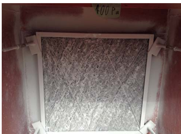
写真-71 圧力損失 400Pa
