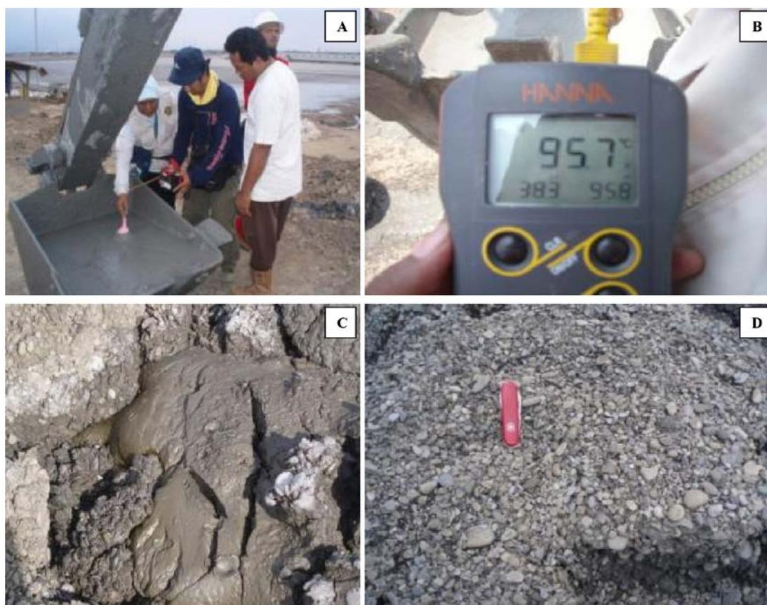
**Fig. 3.** Mud of Lusi composed mostly of water with fragments of shale, silt, andesite, tuff, and various minerals. The temperature of the mud is nearly at boiling temperature. A: Sampling hot mud of Lusi from the crater. B: Temperature ( $^{\circ}\text{C}$ ) of hot mud. C: Dried mud. D: Mud washed by rain.
