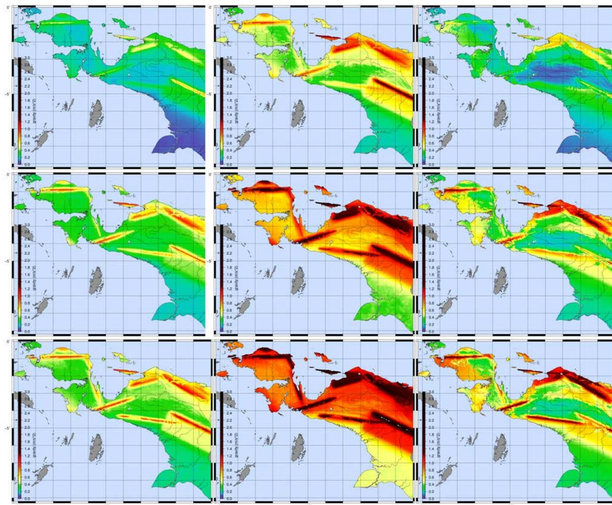
**Fig. 5.** Result of PSHA, first row shown ground acceleration for 100 years return period on 0.0, 0.2 and 1.0 s response spectra respectively, second row and third row shown ground acceleration for 500 and 1000 years return period.
