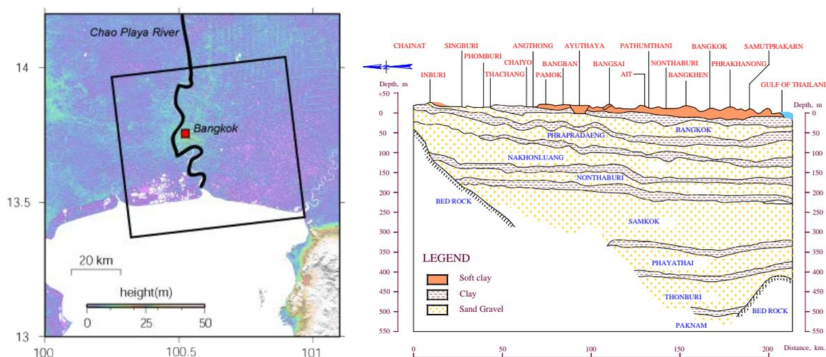
**Fig. 1.** Topography in Bangkok plain and the area of interest (left), and north-south cross section of the hydrogeological setting of the multi-aquifer system beneath Bangkok (right) (Piancharoen, 1997).
