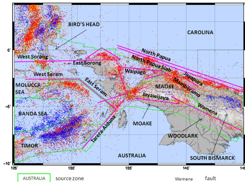
**Fig. 4.** Source zones, fault sources and intraslab source used in this PSHA modeling. The green polyline indicates source zone border, red line indicates fault (include subduction) and intraslab trace.
