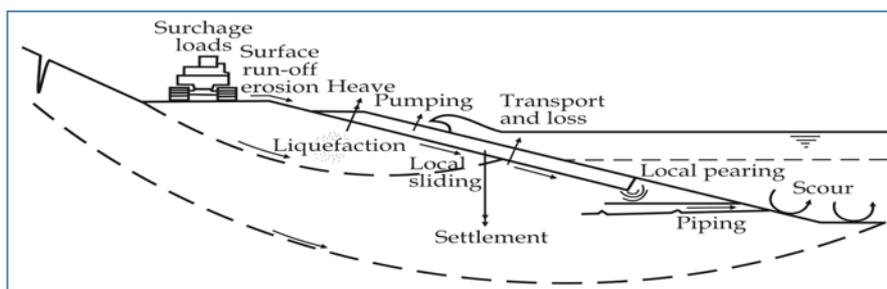
**Fig. 12.** Bank erosion by over-loaded construction model.
