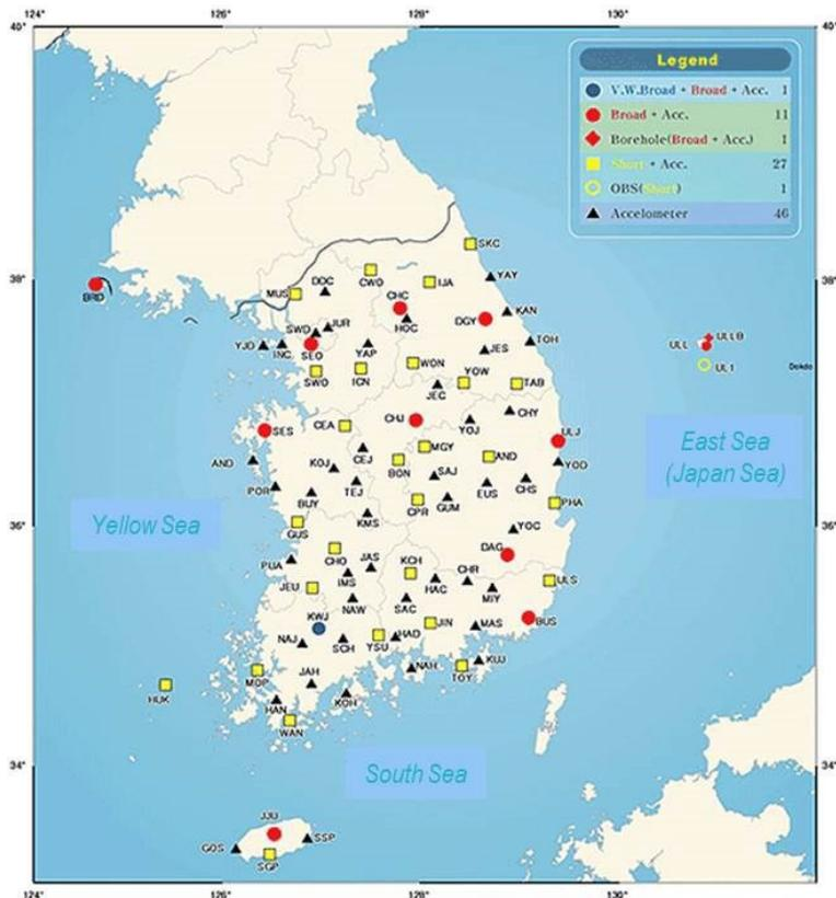
**Fig. 6.** The earthquake and earthquake-generated tsunami monitoring network in Korea which is jointly operated by KMA and KIGAM in Korea (KMA, 2013b). Both agencies are jointly monitoring natural or artificial movements of the earth crust, which are announced by KMA.
