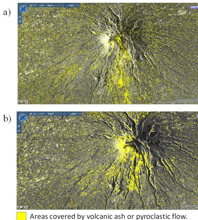
**Fig. 6.** Maps showing the areas affected by the October 2010 Mount Merapi eruptions. a) Map generated using low level feature extraction method. b) Map generated using the frequency based land cover change detection algorithm.
