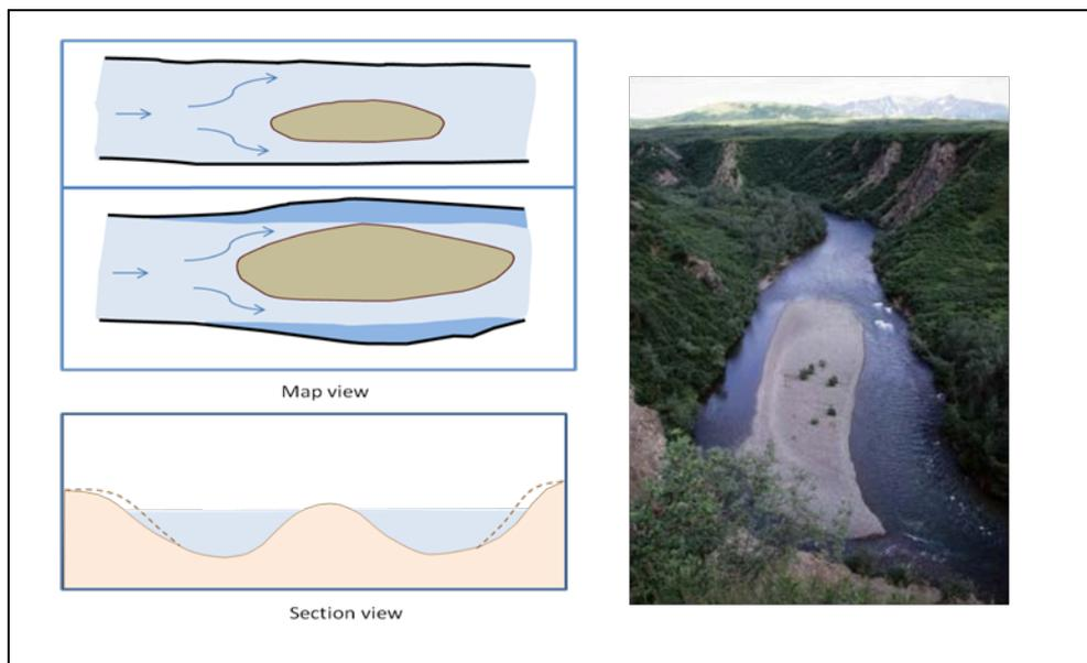
Fig. 5. Riverbank erosion in sand bar area.
