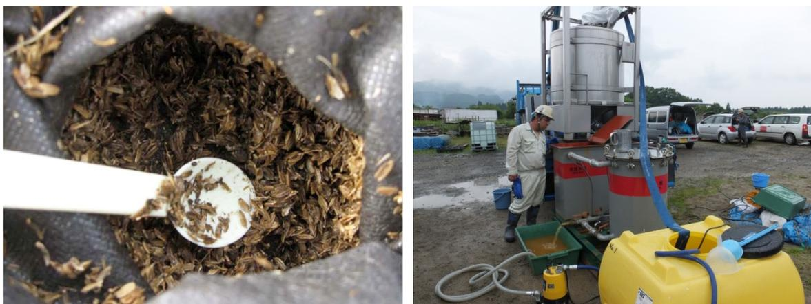
**Fig. 4.** Rice chaff (concentration of more than 30,000 Bq/kg radioactivity) after the test of decontamination of radioactive cesium (left), and a contaminated water purification system using rice-chaff named SEMJ-system (right).
