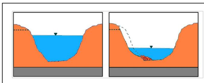
Fig. 9. Riverbank erosion by high differential head.
