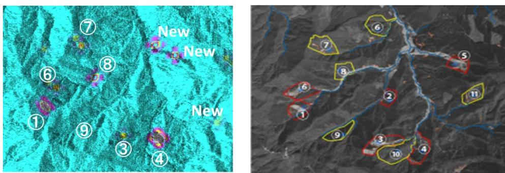
**Fig. 4.** The left side figure indicates the interferogram around the Wanitsuka Mountains of Miyazaki Prefecture (ALOS/PALSAR data acquired from 2006 – 2011). The right side figure shows collapsed area (red) and predicted collapse area (yellow) as was interpreted based on aerial photographs acquired from 1946 to 2005.
