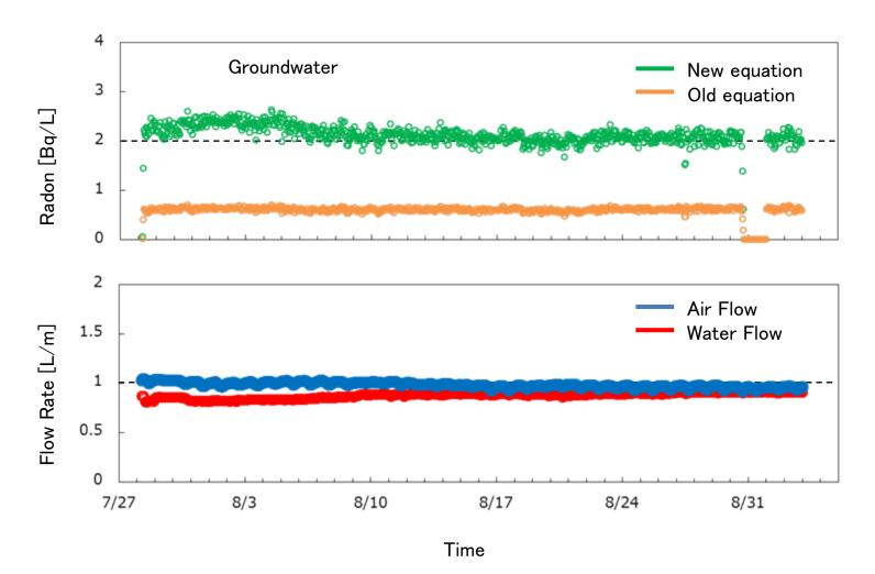
The absolute concentration of radon in groundwater is correctly obtained by the new equation.
