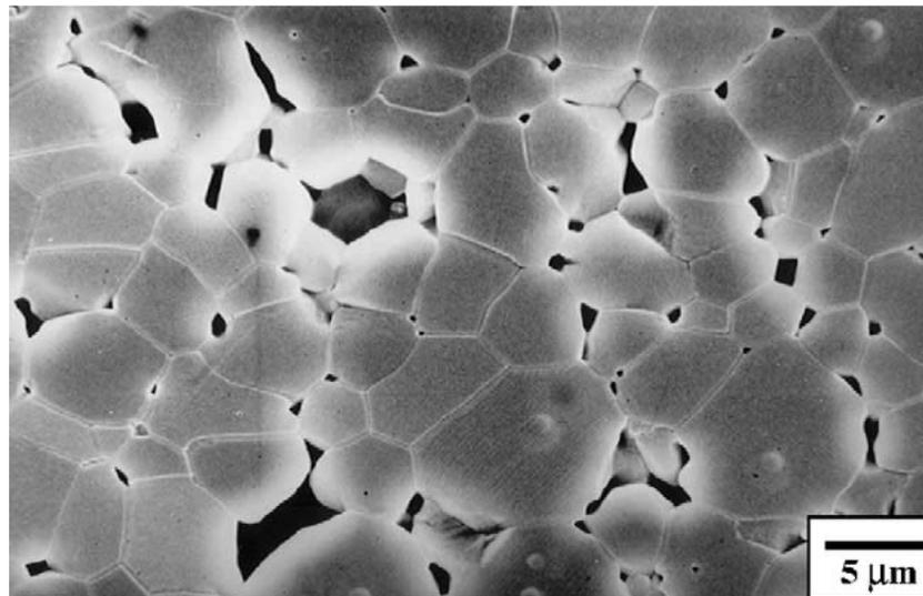
Cavitation during superplastic deformation of alumina
