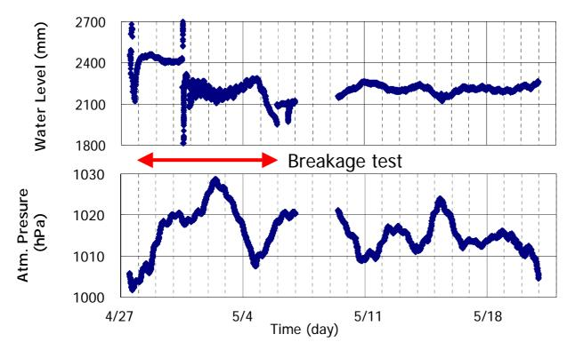
Water level decreased about 30cm after pumping. The value coincides with the volume of the ductwork over groundwater head.
