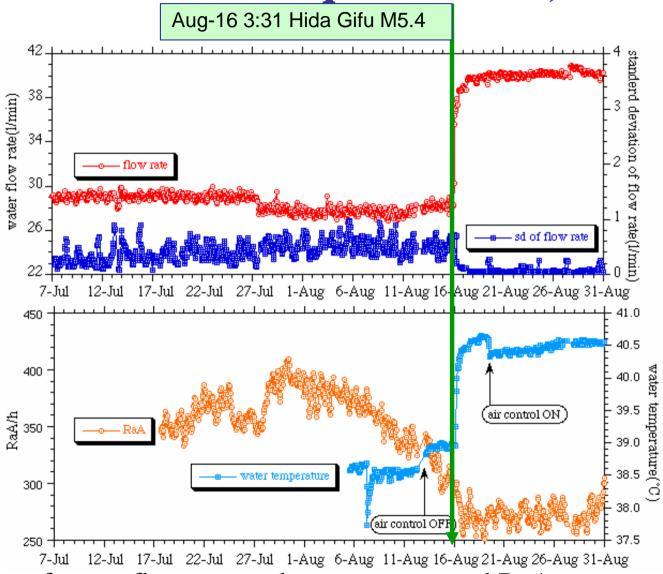
• Decrease of water flow rate and temperature, and RaA counts rate before 3 weeks. Increase of deviation of flow rate before earthquake.
