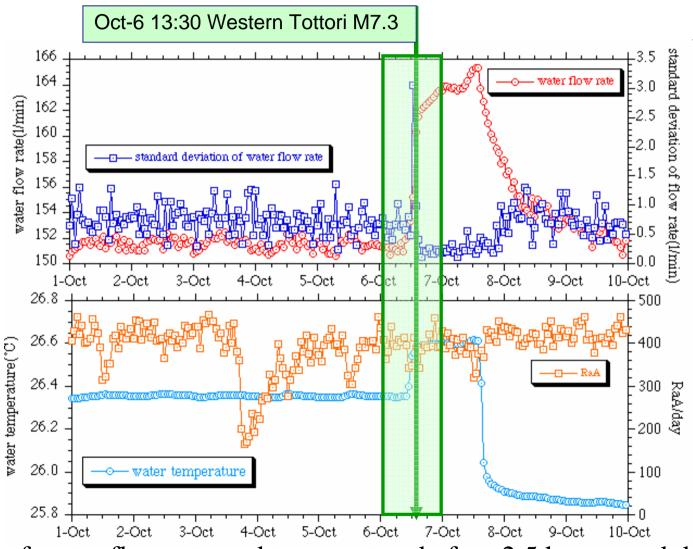
• Increase of water flow rate and temperature before 2.5 hours, and decrease of RaA counts rate. Decrease of deviation of flow rate after earthquake.
