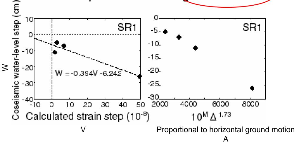
SR1 well: contribution of ground motion seems to be larger than that of strain step.
