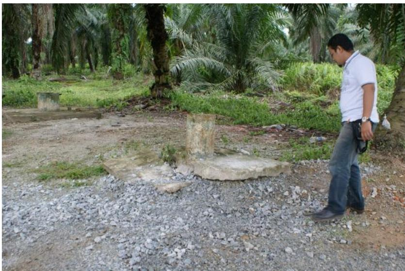
Figure 19: Recent photos showing evidence of ground subsidence within the Langat basin. Photo at the top and bottom showing raised datum point and groundwater well structure relative to the ground surface respectively.
