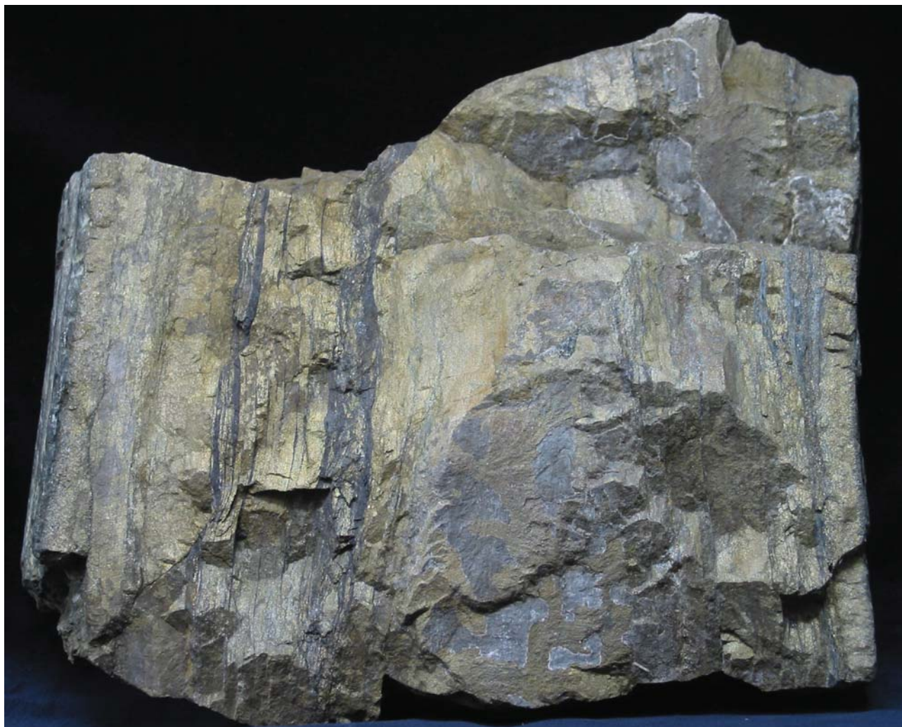
Fig. 2 Laminated pyrite-pyrrhotite-magnetite ore from the Yanahara mine. The magnetic susceptibility vary from 20 \times 10^{-3} (yellow pyrite dominant part) to 268 \times 10^{-3} SI (black magnetite banded part). The samples YAL 4 and 5 (Table 1) are taken from this specimen. Width of the sample is 22 cm. Collection of the Geological Museum of AIST (D33-301).
