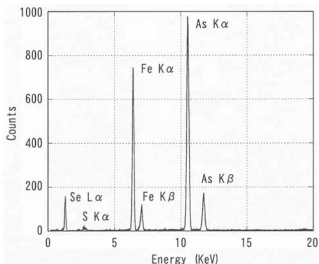
Fig. 4 X-ray spectrum of löllingite obtained with energy dispersive x-ray spectrometer (JEOL JSX-3201).
