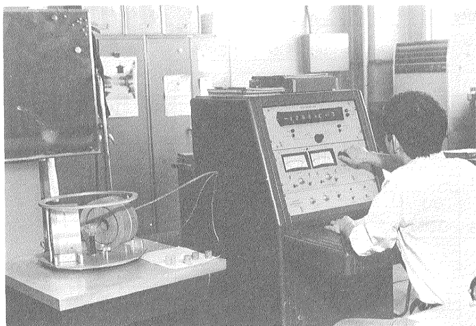
写真5 スピナー磁力計の外観 A view of spinner magnetometer. Left hand: sensor. Right hand: signal analyser.
