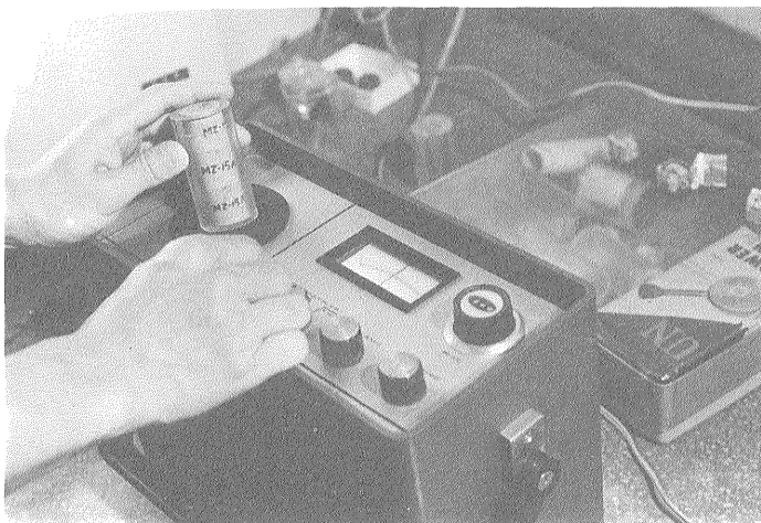
写真4 成形試料の帯磁率測定 Magnetic susceptibility measurements of trimmed rock specimen.
