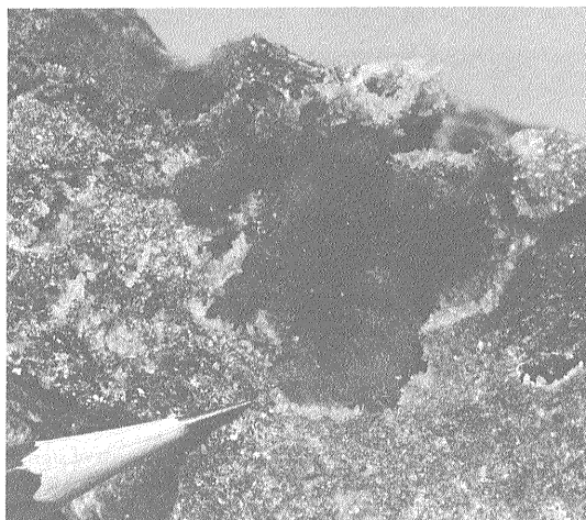
Fig. 16 Occurrence of jamesonite in vugs. Each fibre has a diameter of one to five micron. Tajima vein, —350 m.L.
