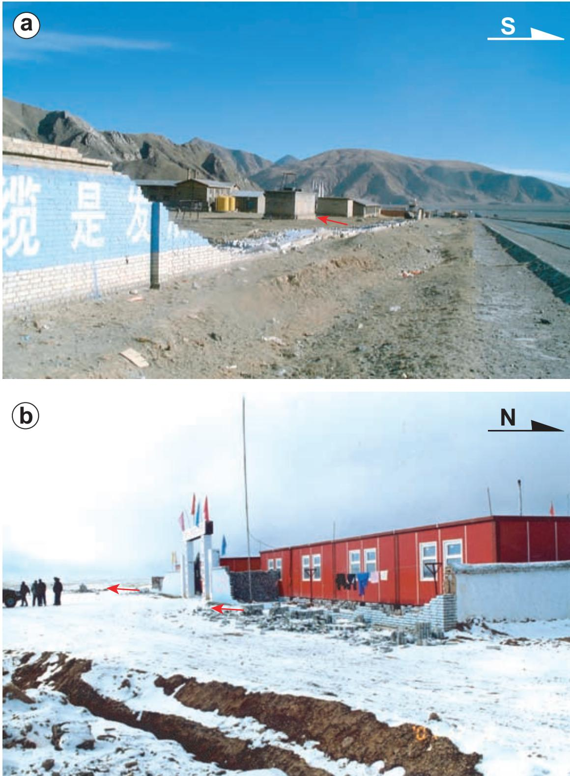
Fig. 12. Walls collapsed during the 2001 Central Kunlun earthquake. (a) A wall fell down toward NNE. Near Xidatan. (b) A wall toppled down toward SSW. 45 km southwest of the Kunlun Pass. Red arrows indicate the direction of collapse.
