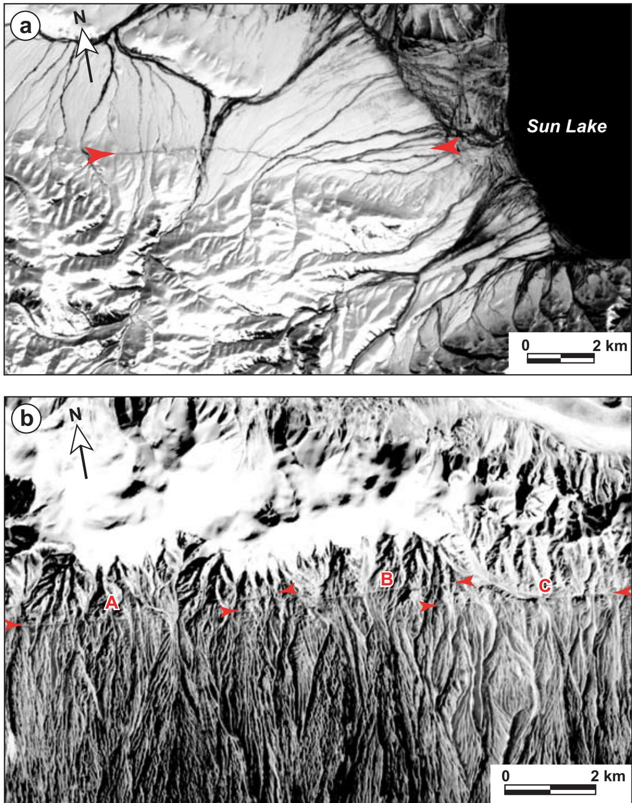
Fig. 2. Satellite images showing the trace of surface rupture zone. (a) Surface rupture zone (indicated by red arrows) appears as a distinctive lineament to the west of the Sun Lake on ASTER image. See Area 1 in Fig. 1b for the location. (b) Coseismic surface ruptures (A, B, and C indicated by red arrows) show a right-stepping en echelon pattern on ASTER image. See Area 3 in Fig. 1b for the location.
