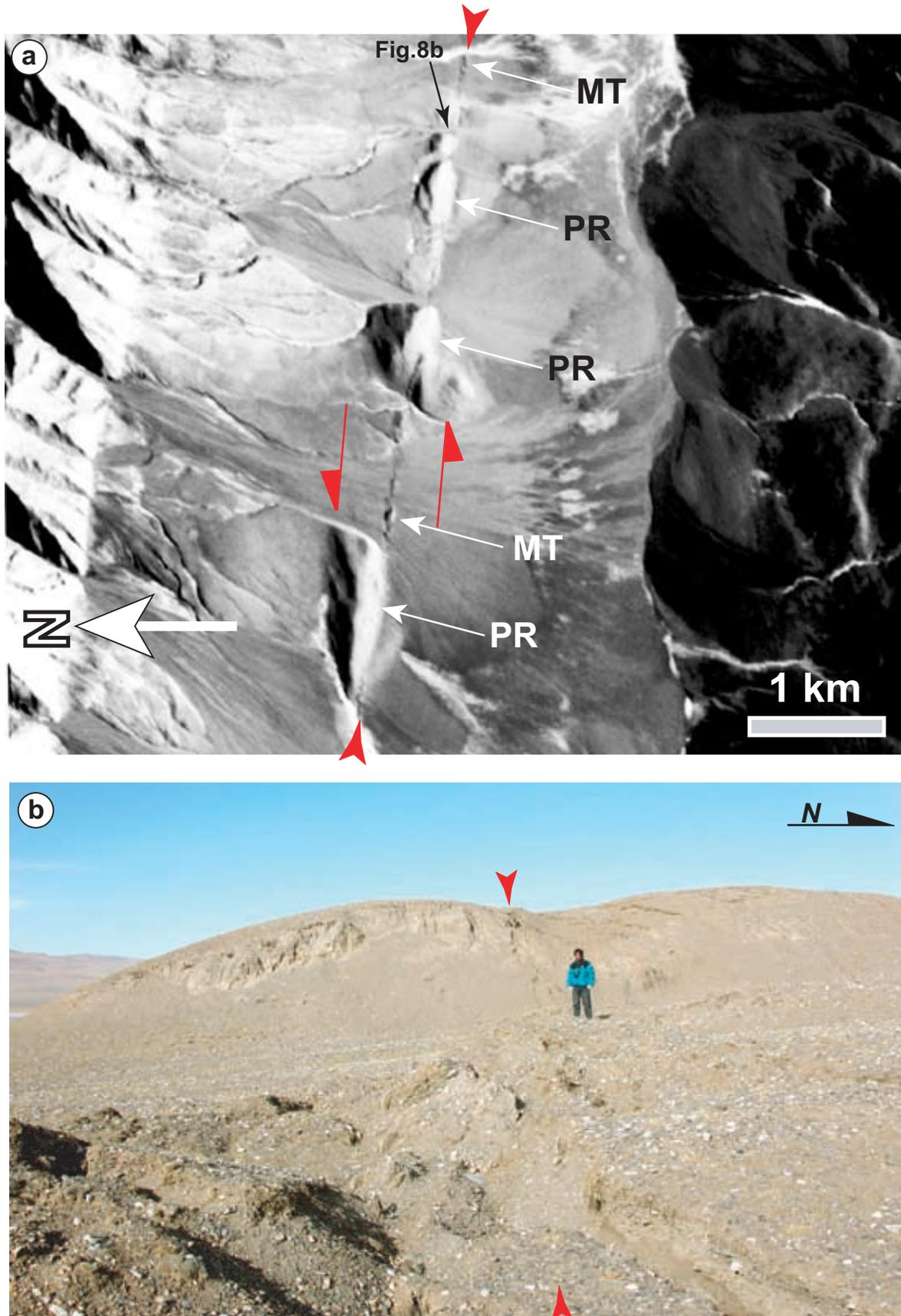
Fig. 8. Large-scale pressure ridges along the Kunlun fault zone. (a) 3D perspective SPOT image shows coseismic mole tracks (MT) and large-scale pressure ridges (PR) to the west of Kusai Lake. See Area 2 in Fig. 1b for the location. (b) A pressure ridge appears as a small hill. Note a coseismic surface rupture indicated by red arrows. See the person for the scale. Location is given in Fig. 8a.
